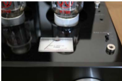
The LM-881A has a bias meter on the top, the more expensive models have one or more meters on the front panel.
