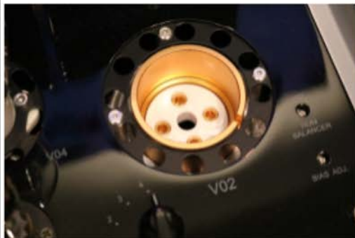
LM-8051A power tube socket. Note the conveniently placed Hum Balancer and Bias Adjust pots.
